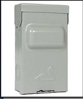
60 amps Non-fused. 240v A.C. Single Phase. UL Listed Three piece construction that opens up mounting and wiring areas, reduces installation time. Terminals approved for 60°C and 75°C wire. Accepts solid 14-8 AWG copper or 12-8 AWG alum., and stranded 14-3 AWG copper or 12-3 AWG alum. Numerous knockouts. Straight-in / Straight-out wiring saves time and money
